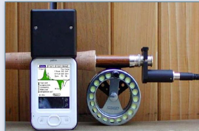
The entire *Fly Casting Analyzer System*: a sensor capsule, a small cable that connects the capsule to the (black) circuit box, the circuit box, and an attached Palm Pilot. A casting signature can be immediately analyzed using the Fly Casting Analyzer software installed on the Palm.
